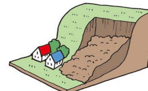
がけ崩れ(急傾斜地の崩壊) Cliff failure (collapse of steep a slope)
